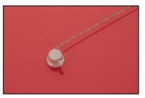
The ferrule is firmly crimped and the cable is cut flush with the end of the ferrule.
