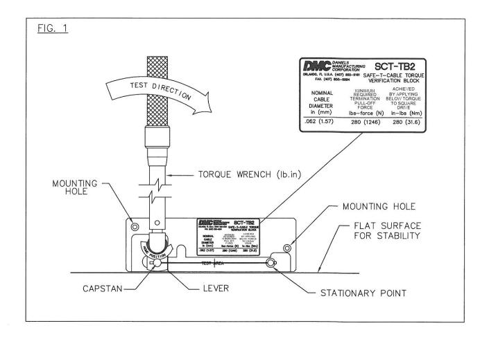
A: Thread the cable into the stationary point and through the capstan, holding the lever in the home position as shown in FIG. 1. Terminate the cable as described in Section 3.0 of ISO336 APPLICATION TOOL INSTRUCTION SHEET, or SCT062—DS Datasheet, making sure to close the handles completely. If the lever is not kept in the home position, the results may be adversely affected.
