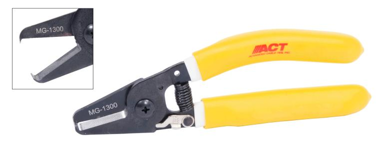
Safely remove cable ties or lacing tape from wire harnesses or cable bundles. This heat treated alloy steel tool has a hooked blade with a safety guard that slides behind the cable tie to prevent cutting or nicking the insulation of the wires. Softly padded and ergonomically shaped handles make the tool comfortable to use and a locking lever keeps the tool closed when it is not in use.
