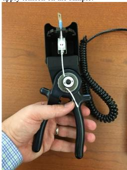
7. After the wire has separated from the termination, the tensile force required for the break can be read directly from the display read out.
