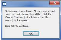
If the instrument is properly connected and configured but this message still appears, the COM port connection may be manually configured. Refer to the communication flowchart below and the following sections for details.
