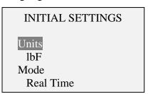
To change Units, scroll to UNITS, press ENTER, and use UP/DOWN ARROWS to change the Units. Press ENTER when desired level is displayed. Press ESCAPE to return to main menu.
