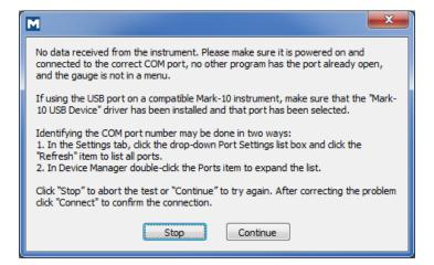
This message appears after clicking **START** if communication has not been achieved between the instrument and the software, due to a number of possible causes. If unable to establish communication based on these instructions, try a different USB / COM port, or a different PC.
