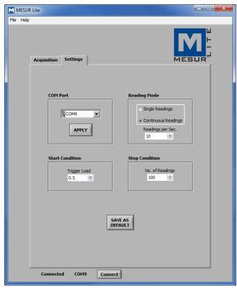
Use this tab to select the PC's COM port number, reading mode, and start and stop triggers. These settings can be saved as default.
