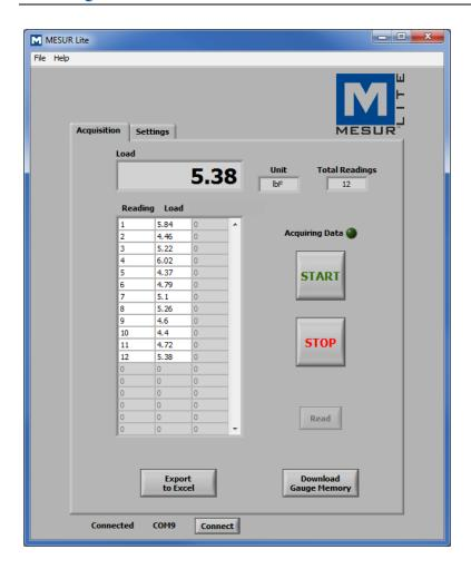
Use this tab to start and stop the test and observe the collected data in tabular format. From this tab, it is also possible to download saved data from a compatible instrument's memory, and also to export data to Microsoft Excel.
