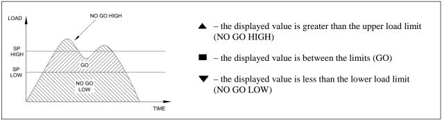
**Note:** Set point indicators and outputs reference the displayed reading, not necessarily the current live load. To return to the MENU screen press ESCAPE.
