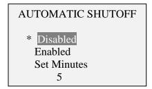
To Disable Automatic Shutoff, highlight DISABLED and press ENTER; an \* will appear next to DISABLED. To Enable Automatic Shutoff, highlight ENABLED and press ENTER; an \* will appear next to ENABLED.
