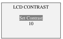
Scroll to SET CONTRAST, press ENTER, and use UP/DOWN ARROWS to change the contrast level. Select a value from 0 to 25, 25 producing the most contrast. Press ENTER when desired level is displayed. Press ESCAPE to return to main menu.
