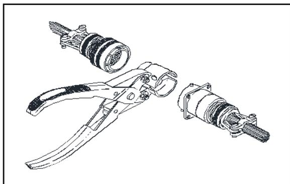
**DMC601 Backshell Tool Kit for Circular Electrical Connectors**
