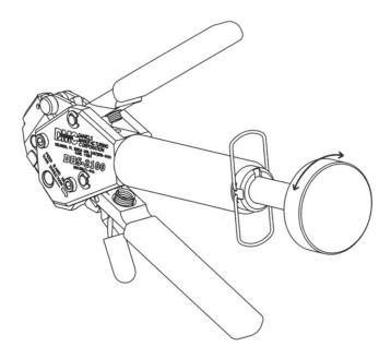
Step 4: Verify the tension applied to the band is within the specified tolerance
