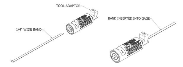
Step 2: Insert the end of the band into the DBS-2100
