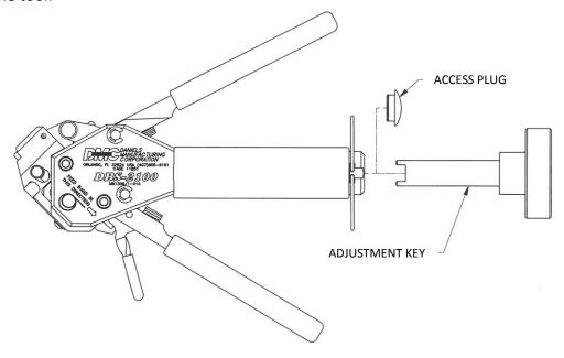
Step 2: Insert the adjustment key into the access hole
