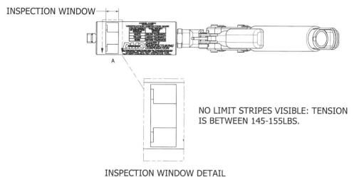
If any amount of the yellow stripe is visible, the tension applied to the band by the DBS-2100 is above 155LBS. This indicates that the tension setting for the DBS-2100 must be adjusted. (See section 1.2 for adjustment instructions.)
