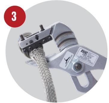
3 Use the rollover tool to roll over the cutoff tab.
