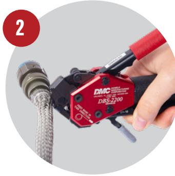
2 Tension the band using the black tensioning handle until the banding tool locks.
