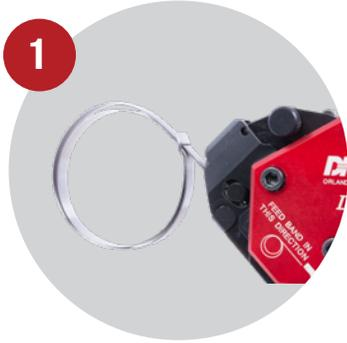
1 Squeeze the release lever to insert the band loop-side down.
