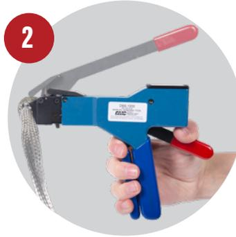
2 Lift the red cutter lever up to secure the band and back down to terminate the band.
