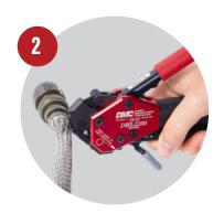
Tension the band using the black tensioning handle until the banding tool locks.
