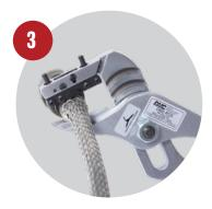
Use the rollover tool to roll over the cutoff tab.
