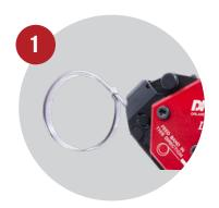
Squeeze the release lever to insert the band loop-side down.
