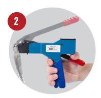
Lift the red cutter lever up to secure the band and back down to terminate the band.
