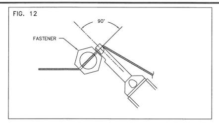
3.10 After crimping and cutting, release the tool handle and slide the tool off the crimped ferrule. Pull the excess cable from the tool.
