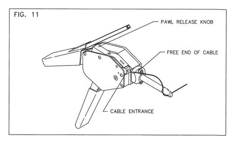
3.8 Begin removing slack from the cable by repeatedly closing the tool handle, allowing the handle to open fully before closing again.
